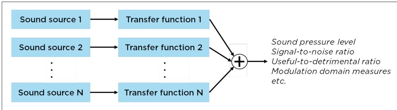
Figure 2. Model description of the Acoustic Scene. The sounds from each of  $N$  separate sound sources are shaped by corresponding transfer functions. As indicated on the output side, the combined sound may be characterized in different ways.
