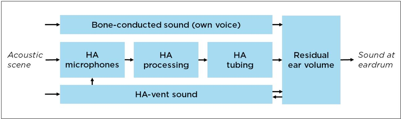
Figure 3. Basic model of the acoustic coupling between Acoustic Scene and Auditory Processing when a hearing aid (HA) is used.
