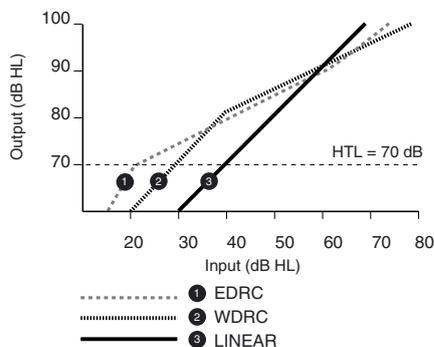
Figure 1. Hypothetical input-output curves of a linear instrument, a WDRC instrument and the EDRC test instruments matched in output for a conversational input level received at the microphone of the instruments worn by a hearing-impaired listener with a 70 dB HL loss.
