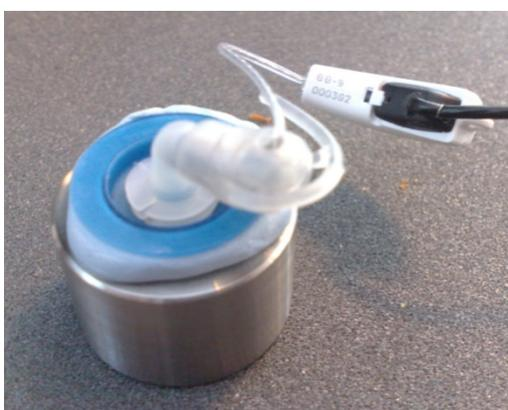
Picture 4: Setup in test box with the hearing aid connected to the HA1 2-cc coupler.
