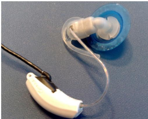
Picture 1: WIDEX BABY440 with Instant ear-tip mounted on the adaptor for the HA1 coupler
