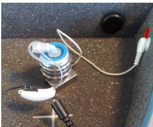
Picture 3: View from the rear of the HA1 coupler. The tip of the ear-tip is flush with the inlet to the coupler volume
