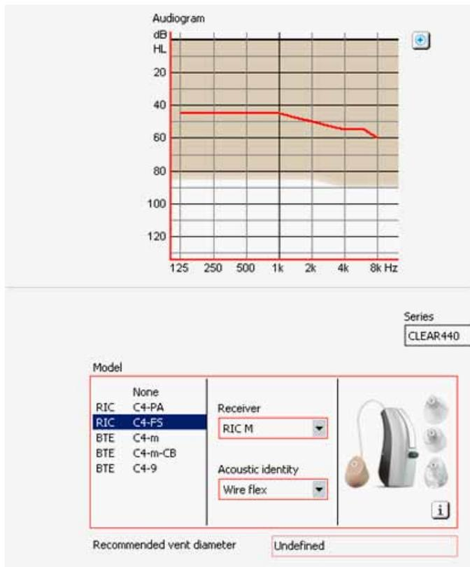
Figur 1. For the hearing loss shown in the audiogram, a FUSION hearing aid with an M-receiver and a Wire flex acoustic identity is chosen.
