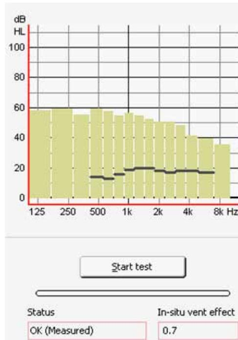
Figure 5. Feedback test using the Instant double (vent: 0.7).
