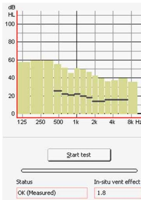
Figure 3. The feedback test, using the Instant tulip ear-tip (vent: Undefined).
