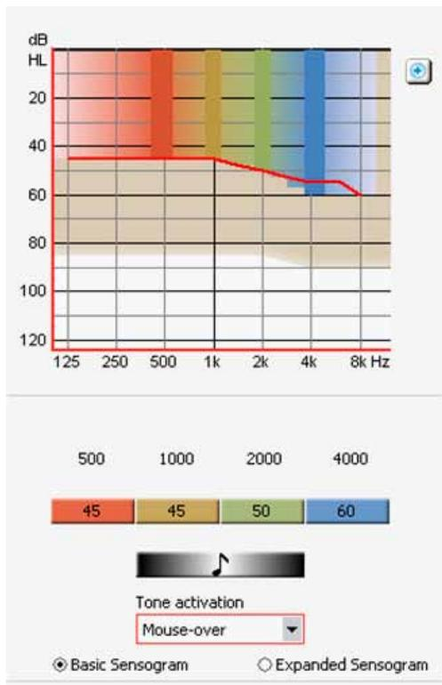
Figure 2. The Sensogram, using the Instant tulip ear-tip (vent: Undefined).
