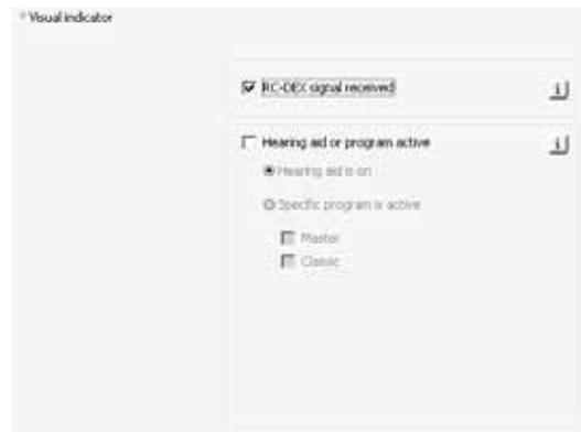
Illustration: The hearing aid can be programmed to flash when a remote control signal is received, when the hearing aid is on, or when a specific listening program is in use.
