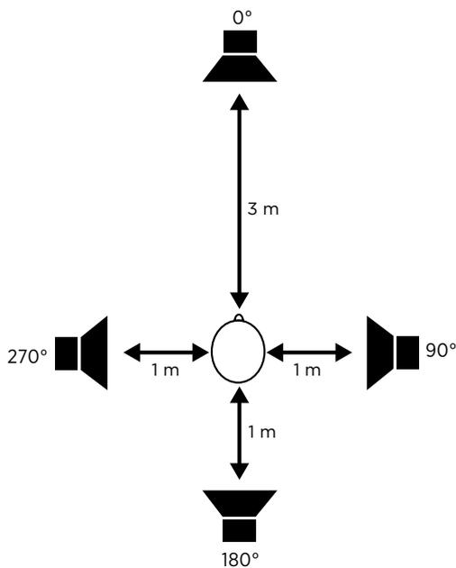
Figure 1: Location of the loudspeakers in the test setup: Loudspeakers were placed in front of the subject (0°), at the rear (180°), to the right (90°) and to the left (270°) at a distance of one and three metres, respectively.
