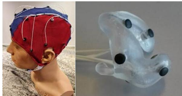
Figure 8. Left: Traditional EEG measurement set-up using a cap with electrodes. Right: Earmould equipped with electrodes used for in-ear EEG. Pictures provided by UNEEG medical.
