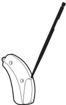
To open battery drawer, use the special tool you've received, and do as illustrated.
