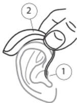
1. Insert the ear-set in the ear while holding the lower part of the tube. Pulling the outer ear upwards and backwards at the same time can be helpful.
