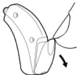
1. Use the nail grip to gently swing the battery door open and remove the old battery.
