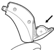
2. Now place the new battery in the drawer as shown. Close the drawer. If it doesn't close easily, the battery is not placed correctly. If you are not using the hearing aid for a few days, remove the battery.
