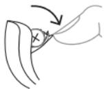
To turn off the hearing aid, pull the battery door downwards.
