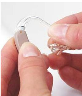
Attach the tube and earmould to the hearing aid.
