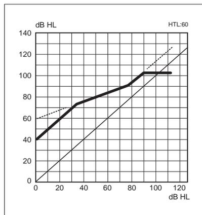
Fig. 10: I/O curve with gain and output limitation.
