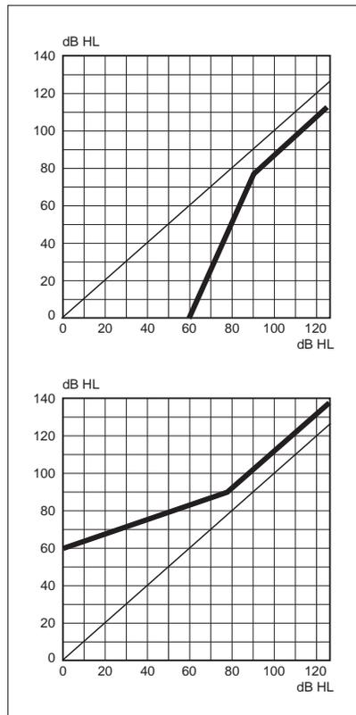
Fig. 9: Loudness template and corresponding input/output characteristic.
