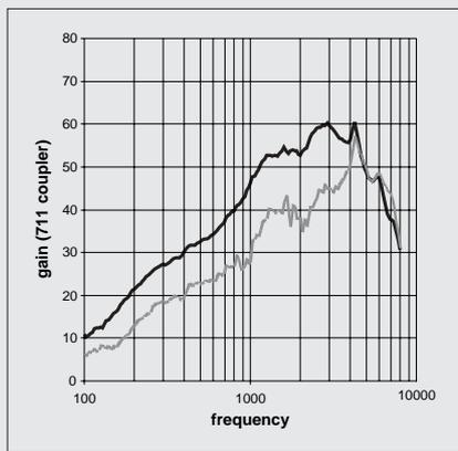
Fig. C.: Front to Back response of the C9.
