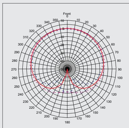
Fig. B.: Free field characteristics for a directional microphone system
