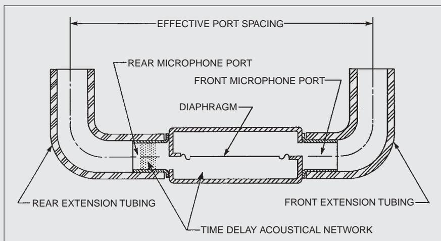
Fig. A.: Dedicated microphone with 2 sound inlets, from Knowles (1989).
