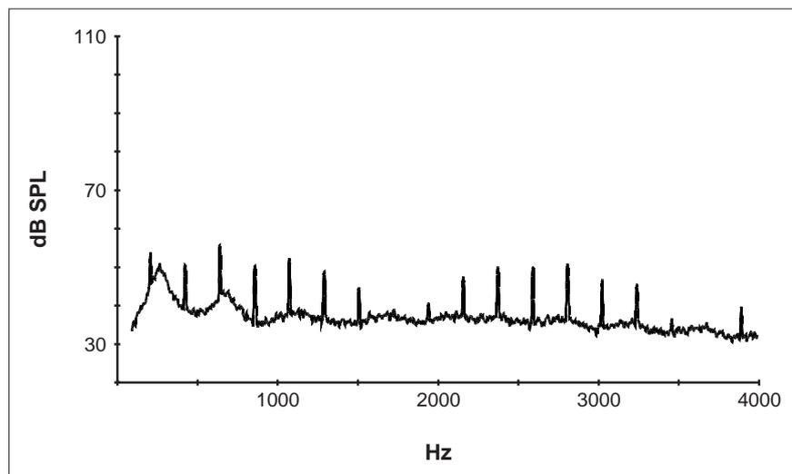
Fig. 8.: Output spectrum of the Widex LOGO hearing aid (model L8, with 2nd generation means to protect against GSM) in the same test condition as Figure 5. Note the significant decrease in output.
