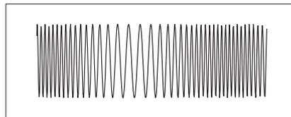
Fig. 2.: FM modulation in analogue cellular phones. The frequency of the carrier is varied according to the proper signal. The amplitude remains constant.
