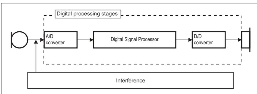
Fig.6.: Block diagram for a digital hearing aid to illustrate the source of interference.
