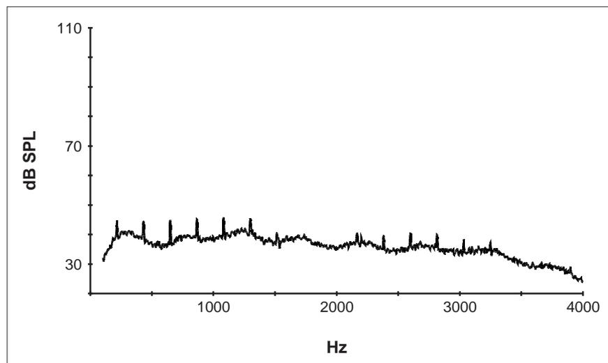
Fig. 9.: Output spectrum of the Widex SENSO hearing aid (model C8, with advanced 3rd generation GSM protection means) in the same test condition as Figure 5. Note that the output has decreased even more.
