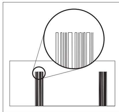
Fig. 1.: Radio signal from GSM cellular phone. 217 times a second a short burst of bits is transmitted.
