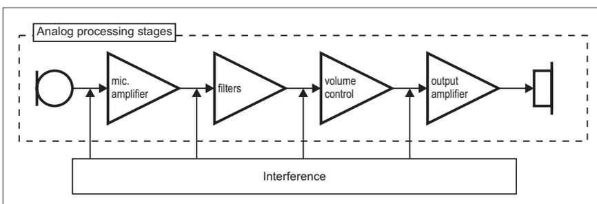
Fig.7.: Block diagram for an analogue hearing aid to illustrate the source of interference.
