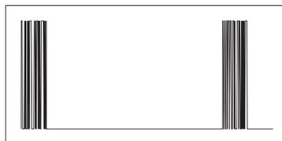
Fig. 4.: AM-like modulation from a GSM phone. Amplitude variations to the high frequency carrier.
