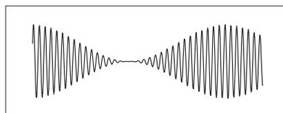
Fig. 3.: AM modulation. The carrier (fast oscillations) has its amplitude modulated with the proper signal.
