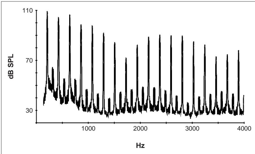
Fig. 5.: Output spectrum from a conventional analogue hearing aid without GSM protection means when a GSM phone is placed next to it. Note the dominant output at 217 Hz. The “spikes” are the harmonics of the modulation frequency.
