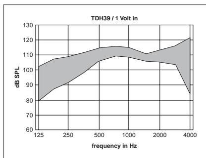
Fig. 1: Range of sound pressures produced by an audiometric earphone mounted in a circumaural cushion on ears of different persons. A constant earphone voltage of 1 Volt has been used (Adapted from Rankovic et al. 1992).
