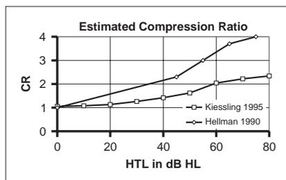
Fig. 3: Compression ratio vs. hearing threshold level obtained from two studies (Kiessling 1995, Hellman and Meiselman 1990).
