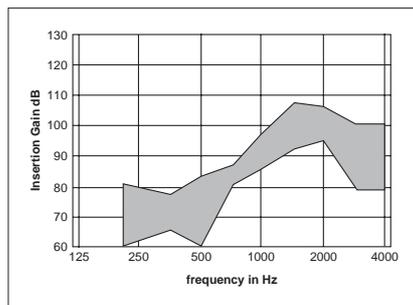
Fig. 2: Range of insertion gains produced by a hearing aid when fitted to the one ear of 17 different subjects (Adapted from Olsson 1985).
