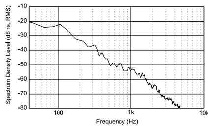
Fig. 4 Spectrum of car noise.
