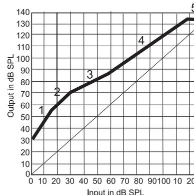
Fig. 2 Example of an input/output curve for the test-HA.
