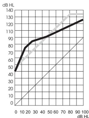
Fig. 3 I/O curves at 500 Hz for the test-HA (black) and for the ref-HA (gray).
