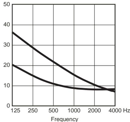
Fig. 4. Equivalent input noise in third octave bands of two similar hearing instruments, one with an omnidirectional microphone (lower curve) and one with a directional microphone (upper curve).
