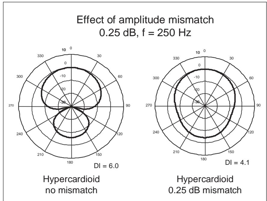
Figs. 2a-b. Directivity pattern at 250 Hz of a directional unit consisting of two omni-directional microphones. Distance between the microphone inlets is 10 mm. a) The internal delay is adjusted to give a hypercardioid pattern with perfect amplitude and phase match. b) Amplitude mismatch of 0.25 dB between microphones.
