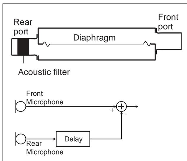
*Figs. 1a-b. Schematics of a) a dedicated directional microphone with the single microphone with two inlets separated by a membrane (adapted from Knowles Electronics, Inc.); b) a directional microphone consisting of two separate cartridges, each containing one membrane and one acoustical input port.*
