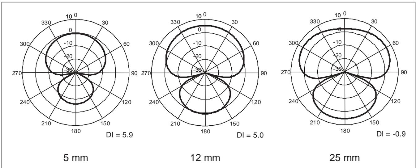
Fig. 6. Directivity pattern at 8000 Hz of a directional unit consisting of two omnidirectional microphones spaced at 5 mm, 12 mm and 25 mm. The internal delay is adjusted to render a hypercardioid pattern with perfect amplitude and phase match.
