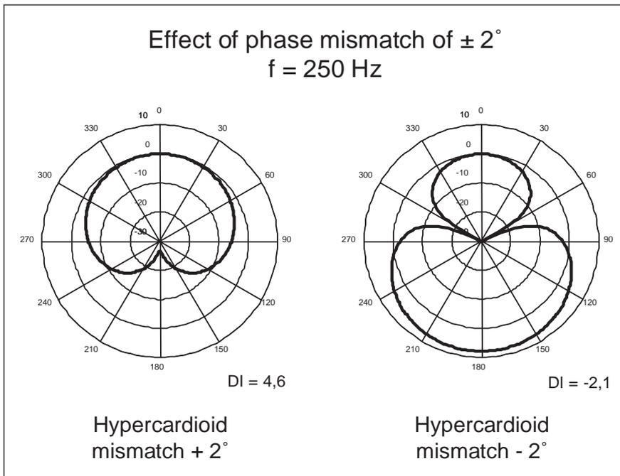
*Figs. 3a-b. Directivity pattern at 250 Hz of a hypercardioid microphone with perfect amplitude match (same as Fig. 2a), except a) phase mismatch of  $2^\circ$  (front microphone is delayed); b) phase mismatch of  $-2^\circ$  (rear microphone is delayed).*
