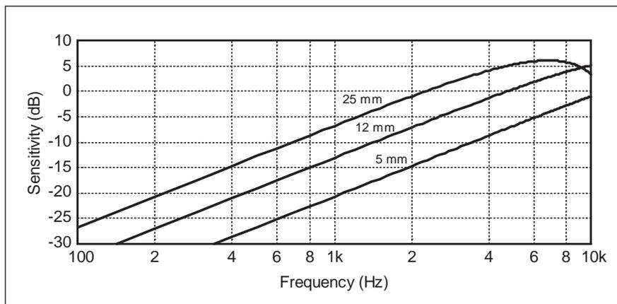
Fig. 5. Effect of port (or microphone) separation on sensitivity in a directional microphone.
