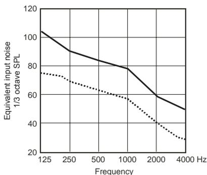
Fig. 7. Wind noise: Equivalent input noise levels measured in third-octave bands for a BTE hearing instrument equipped with a directional microphone (solid line) and an omnidirectional microphone (dashed line). Data from Dillon et al.<sup>15</sup> using KEMAR.
